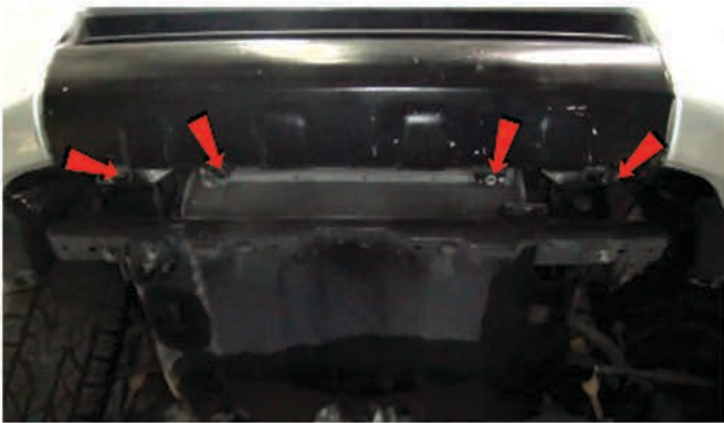
7) Remove [4x] plastic retainers securing the fascia from below.
