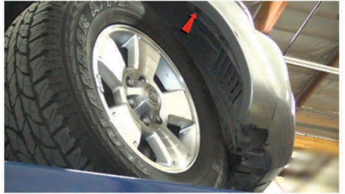
36) Reinstall [1x] plastic retainer to secure the fender liner.
