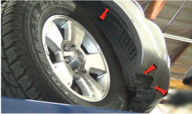
35) Reinstall [3x] phillips screws to secure the fender liner to the fascia.
