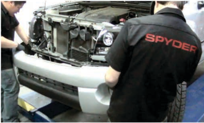
29) Seat the front bumper fascia. Be sure to reconnect the foglight harnesses, if equipped.
