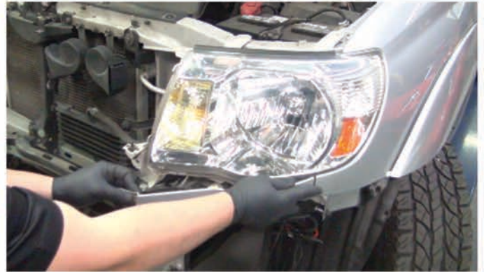
12) Remove the headlight garnish by gently swinging it outwards and away.
