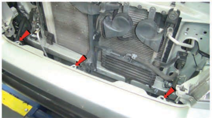
8) Remove [3x] plastic retainers securing the fascia below the grille.
