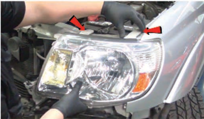
13) Release the headlight retainer tabs.
