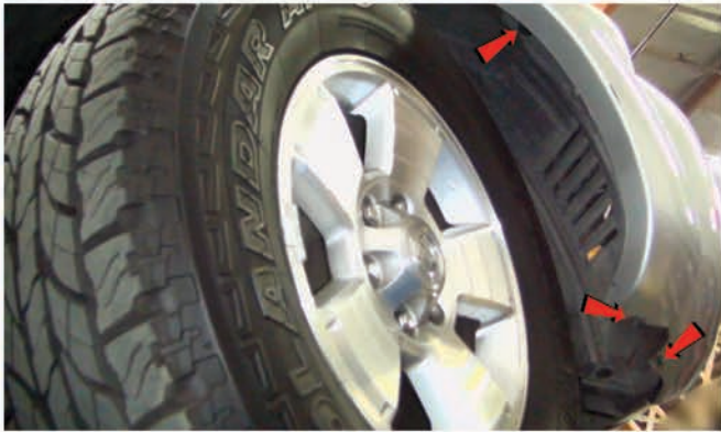
5) Remove [3x] phillips screws securing the fender liner to the fascia.
