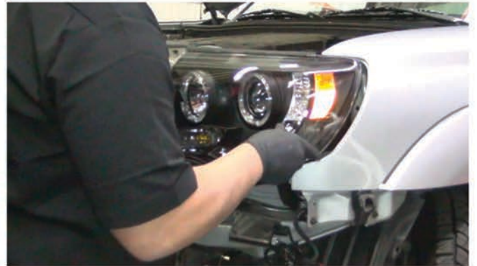
24) Seat the Spyder headlight, being sure to properly seat the headlight retainer tabs.
