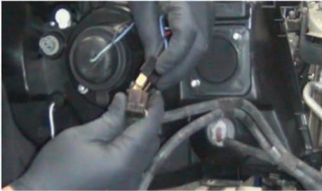
23) Reconnect the headlight harness to the Spyder headlight.
