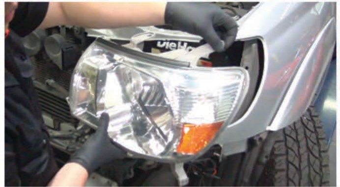
14) Unseat and remove the headlight.
