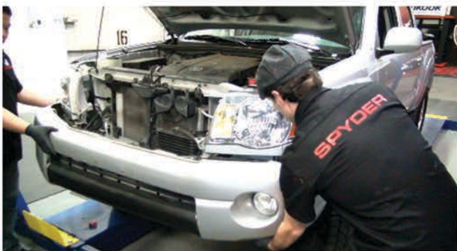
9) Unseat the front bumper fascia. Be sure to disconnect the fog lamp harness if equipped.
