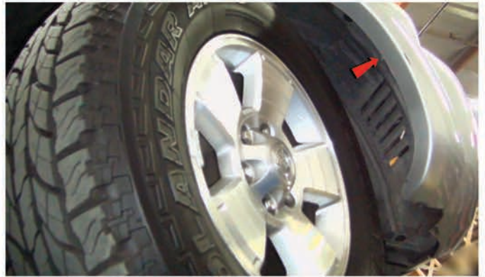
6) Remove [1x] plastic retainer also securing the fender liner, then peel back the fender liner.
