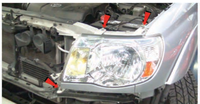
10) Remove [3x] phillips screws securing the headlight.
