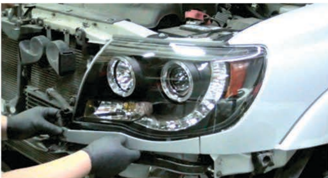
27) Replace the headlight garnish.
