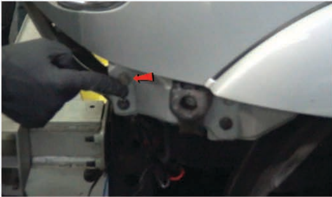
11) Remove [1x] 10mm bolt securing the headlight from the side.
