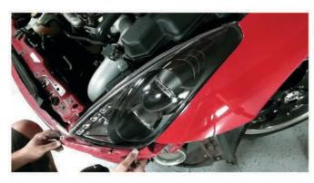
6) Next, seat the head light back onto the frame of the car and screw the (3) bolts back into the mounting holes then replace the head light bracket to support the head light. Replace the (3) bolts for the bracket and secure them all down.
