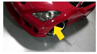
2) Once the bolts have been removed, you will need to move down to the fender liner and remove (1) 10mm bolt on either side of the bumper. Using the 10mm socket, remove them.
