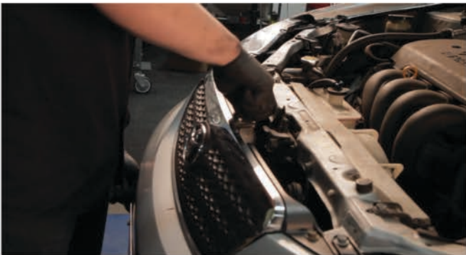
21) Reinstall [3x] 10mm bolts to secure the fascia.
