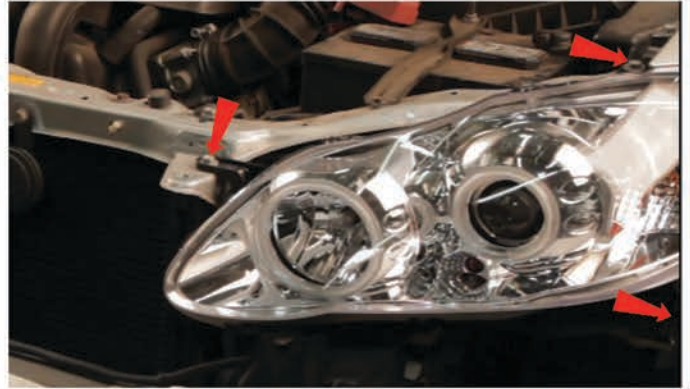
18) Seat the Spyder headlight, then reinstall [3x] 10mm bolts to secure the headlight.
