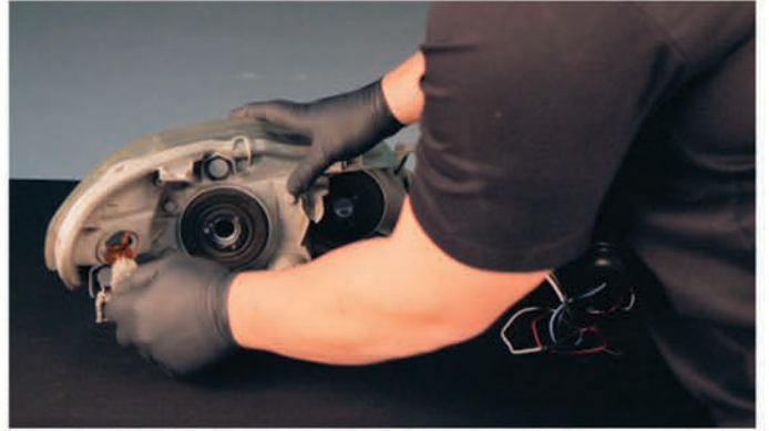
12) Remove the turn signal socket from the OEM headlight.
