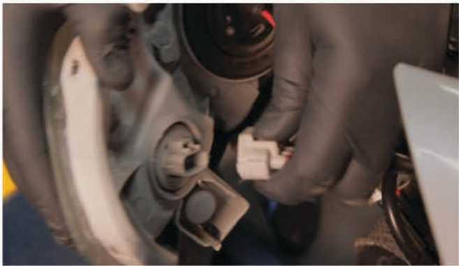
7) Disconnect the turn signal harness.
