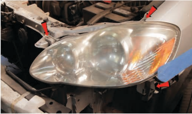
5) Remove [3x] 10mm bolts securing the headlight.
