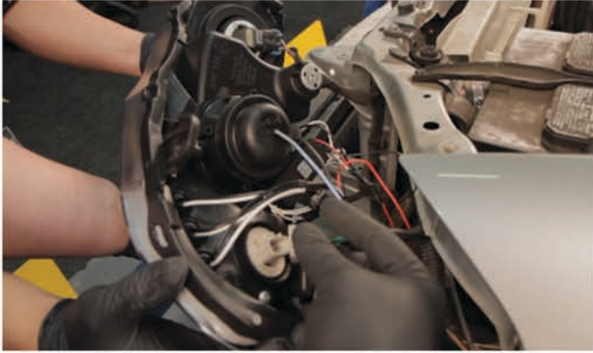
17) Reconnect the turn signal harness.
