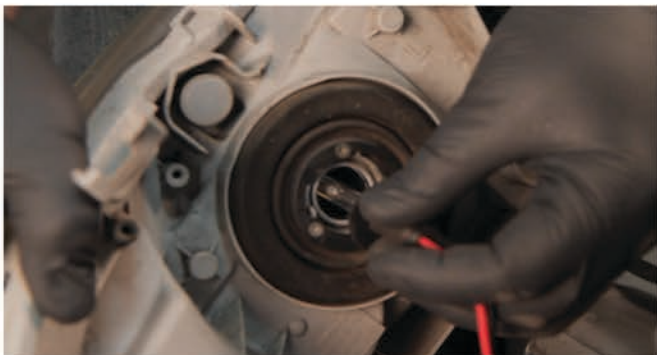
9) Disconnect the low beam harness.
