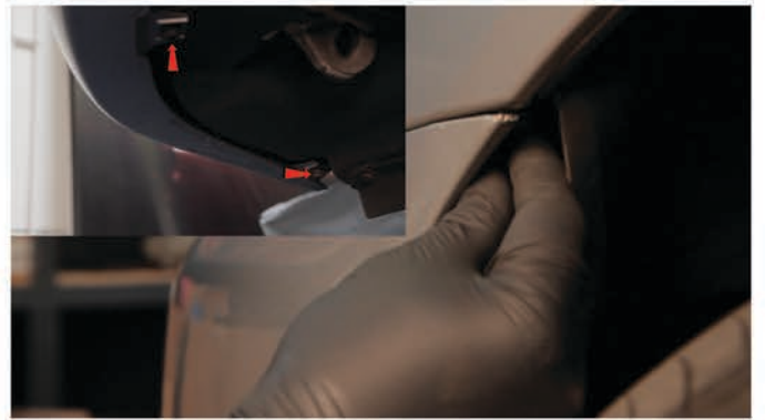
20) Reinstall [1x] 10mm bolt securing the fascia to the fender. Reinstall [2x] 10mm bolts on the bottom corner of the fascia on each side.
