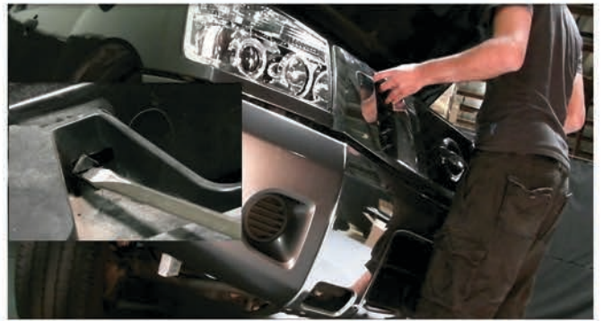
14) Reinstall the grille and reinstall the [7x] Plastic Retainers securing grille by twisting them into place using a flathead screwdriver.
