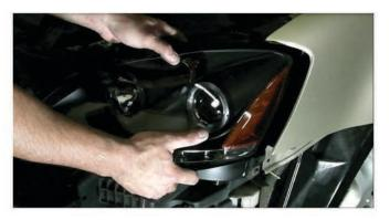
10) Install all bulb sockets into the new SPYDER headlight, then seat the SPYDER headlight after connecting it to the wiring harness.
