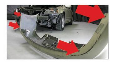
14) Reinstall [4x] 10mm Bolts securing the under side of the bumper fascia to the body. (Bumper shown removed for illustration purposes)
