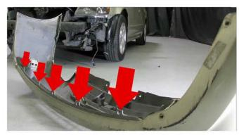
4) Remove [5x] Plastic Retainers securing bumper fascia to body. (Bumper removed for illustration purposes)
