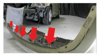
15) Reinstall [5x] Plastic Retainers securing under side of bumper fascia to the body. (Bumper shown removed for illustration purposes)
