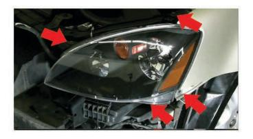
7) Remove [4x] 10mm Bolts securing headlight.
