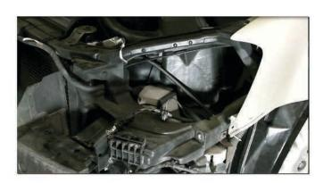
9) <u>Disconnet the headlight by removing</u> all bulb sockets from the OEM headlight, then remove the OEM headlight assembly and set it aside.
