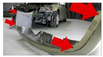
3) Remove [4x] 10mm Bolts Securing Underside of Bumper Fascia to body. (Bumper removed for illustration purposes)
