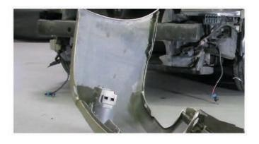
5) Remove the fog light bulb sockets or disconnect the fog light harness [if equipped]. (Bumper removed for illustration purposes)
