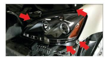
11) Install [4x] 10mm Bolts to mount and secure SPYDER headlight.
