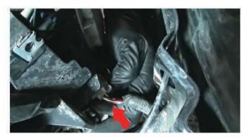
5) In order to remove the head light you will need to disconnect the wiring harness from the bottom of the head light. Pinch the clip to release it from its socket.
