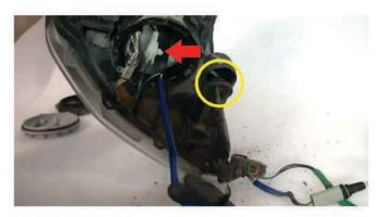
10) Start pulling out the wiring harness until you have reached (2) white sockets clipped together. Remove the sockets from one another to enable the full release of the wiring harness. Next, unseat the rubber seal attached to the head light and pull the entire harness free, seal is shown circled above.
