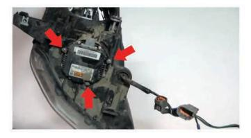
8) Turn the head light over and locate the ballast.Using your Phillips screw driver, unscrew the (3)Phillip type screws to remove it.
