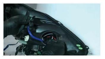
16) Next you will need to open the high beam housing by removing the rubber capping. There will be a small connection wire inside, taking the blue wrapped wiring from the harness previously inserted into the head light, connect the two together and then replace the rubber seal.
