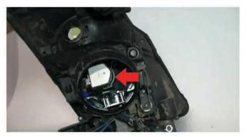
11) Next, the HID bulb and igniter pack will need to removed from the head light. Begin by removing the igniter pack off of the HID bulb. Next, unclip the HID bulb and remove it. Be sure your fingers do not come into contact with the bulb as this can cause the bulb to blow out when reinstalled.
