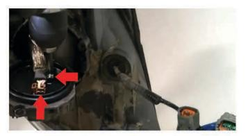
9) Once you have unseated the ballast, you will need to unscrew (1) Phillip type screw then disconnect the igniter pack harness. The clip may be a little hard to pinch, use the tip of the panel popper to assist in removing the clip.
