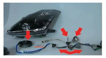
12) Here you will notice all parts removed from the original head light. From left to right: HID ballast, mount screws, HID bulb, igniter pack and wiring harness.
