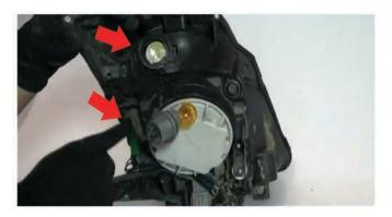
6) Next, you will need to transfer several components to your new Spyder head lights. Begin by removing the complete wiring harness. Unseat all bulbs and sockets top to bottom.
