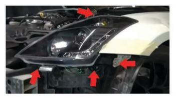
18) Next, replace the (4) 10mm bolts securing the head light to the frame. Place the bumper support foam back onto the vehicles support brace as removed.
