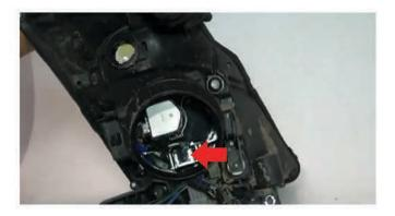
7) In order to reach the harness from inside the head light, unscrew the projector housing cover off. Next, unclip the harness beside the igniter pack as shown.
