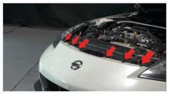
19) Seat the bumper back onto the vehicle and replace the (6) plastic fasteners on top to secure the bumper back to the frame.
