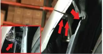
2) Next, you will need to remove (3) 10mm bolts from the fender well, pull back the fender liner to locate them. (1) bolt will be offset from the two and can be seen a bit further back as shown.
