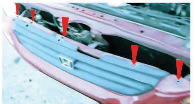
16) Re-seat the bumper fascia and reinstall the five 10mm bolts securing the upper bumper fascia.
