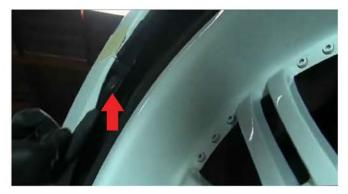
2) Next, there is (1) Phillip type screw that secures the bumper to the fender. Using the Phillips screw driver, remove that screw. This step will need to be done to both driver and passenger sides of the bumper.
