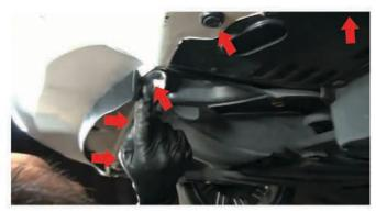
9) Seat the bumper on the vehicle by lining up all mounting holes to their designated bolt holes. You may need to give the bumper a few light taps along the head light to seat it properly. Now that you have seated the bumper replace the bottom (10) plastic fasteners. Be sure they snap into the bumper securely locking it to the frame.
