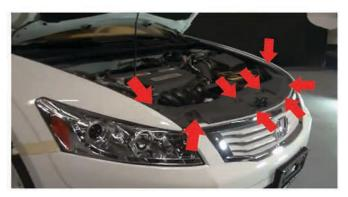
11) Lastly, replace the plastic radiator plate back onto the bumper grill and snap the (8) plastic fasteners back into their mount holes. This should secure the plate and bumper back to the frame.
