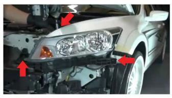
4) Now that the bumper has been removed it is time to <u>unseat the head light</u>. There are (3) 10mm type bolts that secure the head light down to the frame, locations are shown by arrows. Using the 10mm socket and ratchet, unscrew the (3) bolts from the head light and set them aside.
