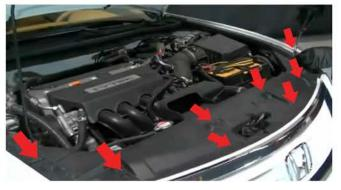
1) The bumper will need to be removed for the head light installation. Begin by opening your hood, locate the (8) plastic fasteners that secure the radiator plate and bumper to the frame. Using the panel popper, pry the fasteners free and set aside for later use.
