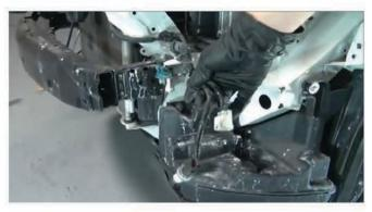
5) Before the head light can be taken off, all sockets must be unclipped from the back housing of the head light. You will need to leave the signal bulb attached to its socket on the harness, this will be placed later in your Spyder head light housing.
