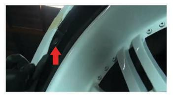
10) Next, move up to the fender lining, replace the Phillip type screw to secure the bumper to the fender.
