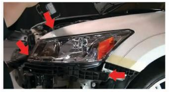
8) Once you have all wiring connected, seat the head light onto the vehicle lining up the mounting holes with the bolt holes on the frame. Replace the (3) 10mm bolts to secure the head light down to the frame. Now you are ready to seat the bumper.
