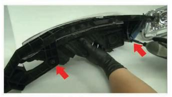
6) Next, once the head light has been removed you will notice it contains a bracket that helps seat the head light to the frame, this will need to be removed and installed on your Spyder head lights. Using the 10mm socket remove the (2) 10mm bolts, place the bracket on the new head light and secure it down with the (2) 10mm bolts previously removed.
