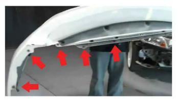
3) Before the bumper can be fully removed from the vehicle there are a total of (10) plastic fasteners (5) on each side of the bumper, remove them with the panel popper. Once removed gently pry the edges of the bumper from the fenders to remove it.
