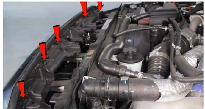
2) Remove [5x] plastic retainers securing the grille.
