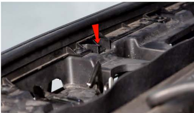
3) Remove [1x] 10mm bolt securing the grille.
