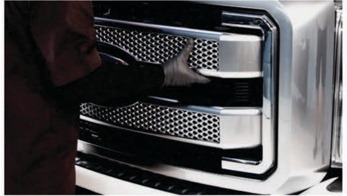
17) Seat the grille, being sure to seat the grille fully into its [5x] retaining clips.
