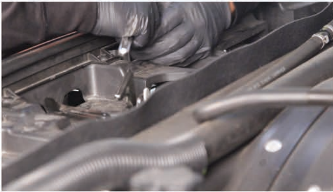
18) Reinstall [1x] 10mm bolt that secures the grille.
