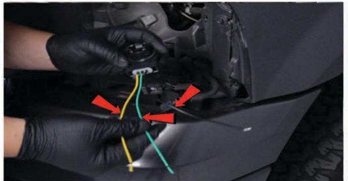
10) On the Spyder turn signal socket, the black wire is ground, the green wire is park lamps and the yellow wire is turn signals.
