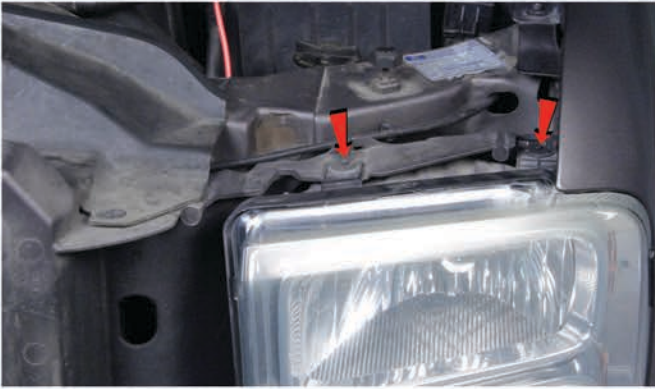
5) Remove [2x] 5.5mm bolts securing the headlight.
