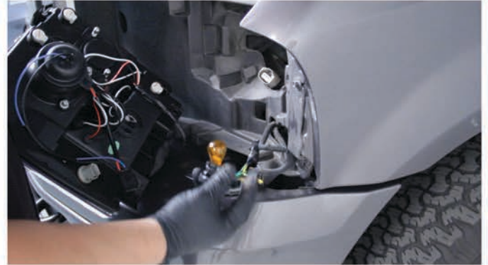
14) Reinstall the turn signal socket.
