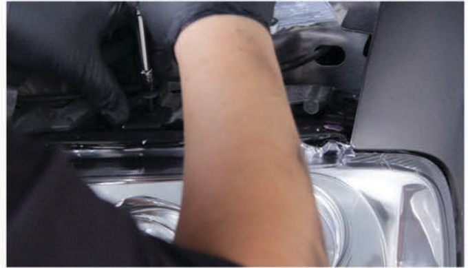
18) Reinstall [2x] 5.5mm bolts to secure the headlight from above.
