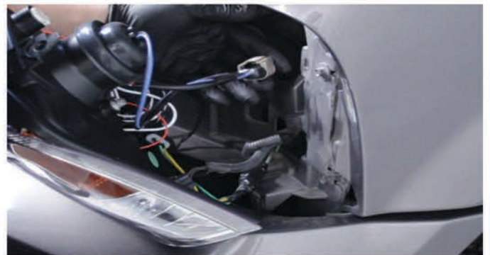
16) Reconnect the headlight wiring harness.
