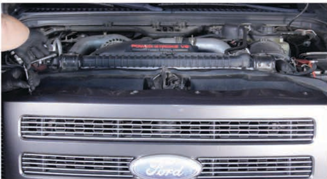
21) Reinstall [4x] 5.5mm bolts to secure the grille.
