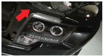
1) Open your hood and locate the plastic Phillips screw that is <u>holding the headlight shroud</u>. Once the plastic Phillips screw has been removed with a Phillips screw driver, fold the shroud back to access the (3) 10mm bolts.
