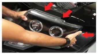
3) Next, gently pull outwards from the back of the headlights to get it free. Still attached will be (3) headlight harness. Disconnect the light harness while retaining the side marker light and turn signal light bulb(will be reused later) which will come out by turning them counterclock wise. Set OEM assembly aside.
