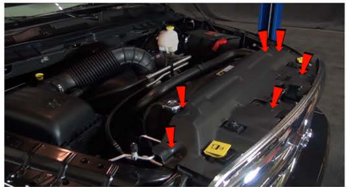
2) Remove [6x] plastic retainers securing the filler panel.
