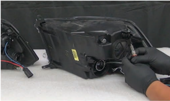
11) Remove the high beam bulb from the OEM headlight. Never touch exposed bulbs with bare hands.
