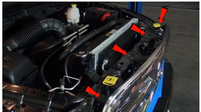
4) Remove [4x] 10mm bolts securing the grille.
