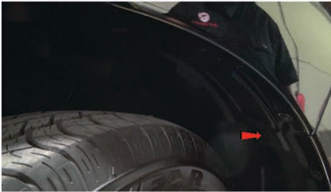
19) Close the access flap, then reinstall the plastic retainer to secure it.
