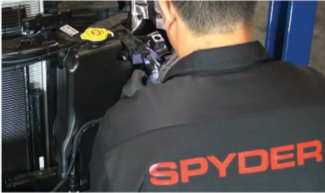
17) Reinstall [2x] 10mm bolts to secure the headlight.
