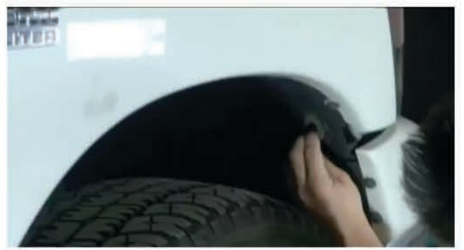
12) Reinstall the fenderwell access plug.
