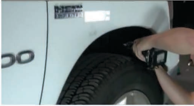
11) Reinstall the 10mm nut that secures the headlight from behind through the fenderwell access hole.
