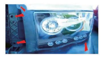
8) Reinstall the three 10mm bolts that secure the headlight and then reinstall the phillips head screw that secures the headlight weatherstrip.
