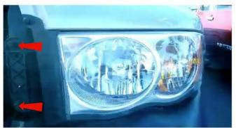
1) Open the hood. Remove the two 10mm bolts securing the headlight.
