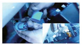
6) Locate your SPYDER headlight. Connect the SPYDER headlight harness to the headlight bulb socket. Install the turn signal socket into the SPYDER housing.
