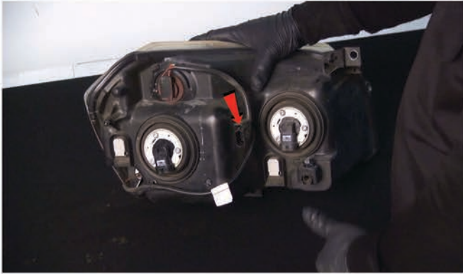
11) Remove the harness connector from the OEM headlight.
