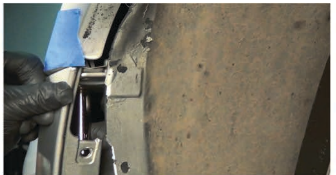
22) Reinstall [2x] 10mm bolts & [1x] plastic retainer at the wheel well to secure the fascia.
