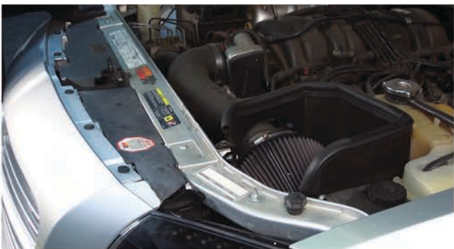
21) Reinstall [6x] plastic retainers to secure the fascia.
