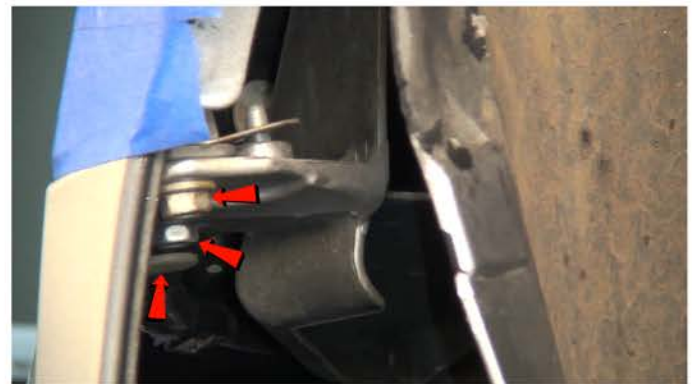
4) Remove [2x] 10mm bolts & [1x] plastic retainer securing the fascia to the fender.
