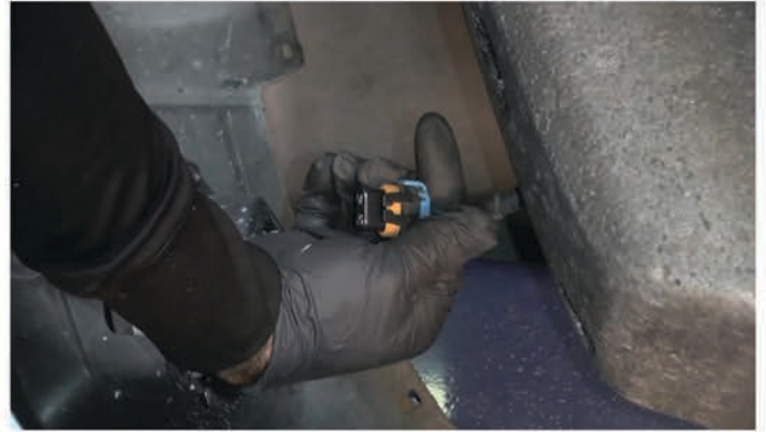
6) Disconnect the fog light wiring harness.
