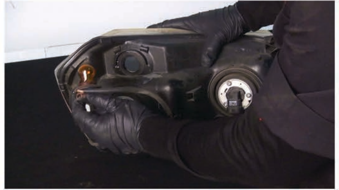
12) Remove turn signal socket from OEM headlight. Never touch exposed bulbs with bare hands.
