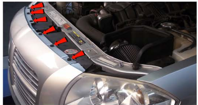
2) Remove [6x] plastic retainers securing the fascia.
