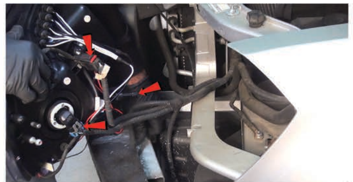
16) Connect the high beam harness, low beam harness and turn signal/park lamp harness to the Spyder headlight.
