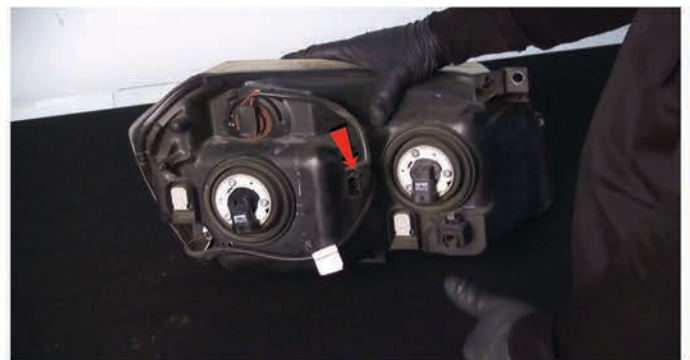
10) Remove the harness connector from the headlight.
