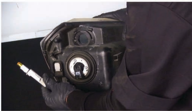
13) Remove the sidemarkers socket, then set the harness aside.
