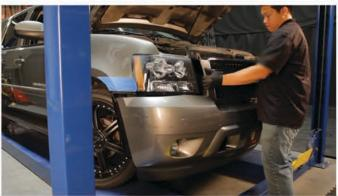
6) Tape off the fender edge to protect the paint while removing and reinstalling the fascia, then unseat the front bumper fascia.
