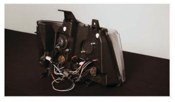
13) Transfer the harness to the Spyder headlight. Connect the high beam harness and low beam harness and reinstall the DRL, turn signal and sidemarker sockets. Your Spyder headlight is now ready to install.
