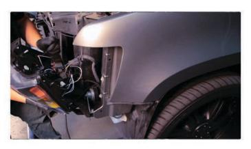
14) Connect the Spyder headlight harness to the main wiring harness.
