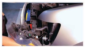
10) Disconnect the headlight wiring harness and remove the headlight.
