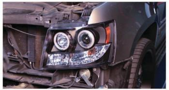
16) Reinstall [3x] 10mm bolts to mount the headlight.
