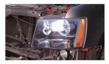
8) Remove [3x] 10mm bolts securing the headlight.
