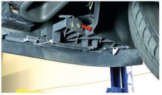
5) Remove [1x] 10mm bolt securing the fascia from below on each side.
