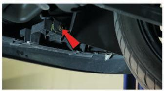
21) Reinstall the 10mm bolt to secure the fascia from below on each side.
