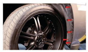
20) Replace the fender liner and reinstall [3x] plastic retainers and [2x] 7mm bolts to secure the liner.
