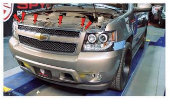
19) Reinstall [6x] 10mm bolts securing the front bumper fascia along the header panel.
