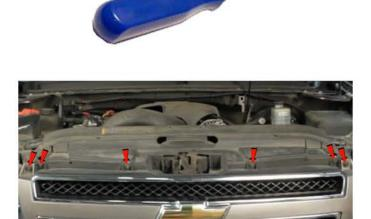
2) Remove [6x] 10mm Bolts securing the bumper fascia along the header panel.
