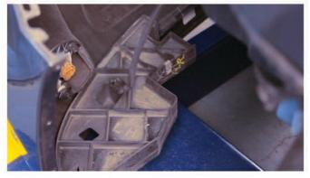
7) Be sure to disconnect fog light harnesses, if your Suburban is equipped with fog lights. Remove the fascia and set it aside.
