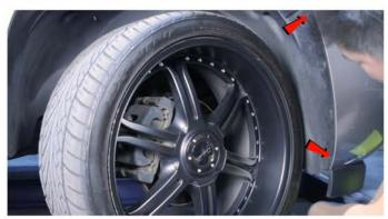
4) Remove the [2x] 7mm bolts securing the fender liner.
