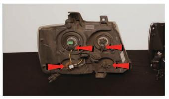
11) Disconnect the high beam and low beam harnesses, then remove the turn signal, sidemarker and DRL sockets. Never touch exposed bulbs with bare hands.
