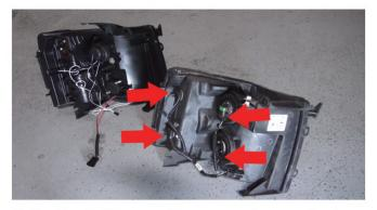
7) Set the OEM assembly next to the new Spyder light. You will need to transfer the bulbs and wiring harness over. The first set of red arrows (left) are your signal/running lights. Turn counter-clockwise to get them free. The second set of arrows (right) will be your bulb harnesses. These can be pulled out fairly easily.
