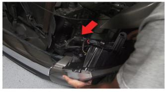
9) Once the wires have all been connected, reattach your OEM harnesses together and mate the connection. Reinstall all panels, bolts, and fasteners in reverse order as shown in steps (6,5,4,3,2,1).
