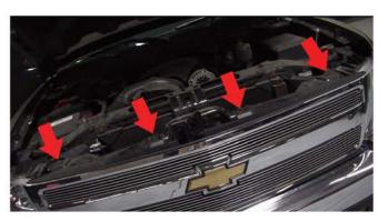
2) Once the bolts have been removed, you will need to remove (4) 10mm nuts, shown here. Once these are out, you will need to unmount the tabs holding the grille in place. They are located directly in front of the radiator support and behind the grille. (fig.3)
