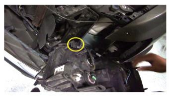
6) Now that all the bolts have been removed, you should be able to get the headlight free. However, still attached to the headlight will be the harness (circled here). Disconnect this harness and now the headlight will fully detach from the vehicle.
