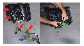
8) Now once you have the headlight harness removed from the OEM headlight set, you will now need to plug it into the new Spyder headlight. Match the like arrows to their sockets and repeat for all bulbs and sockets. Red arrows indicate the running/turn signal bulbs, the blue arrows (orange oem harness to white/blue harness) are your low beam wires, and the green arrows (red oem harness to red/black harness) indicate your high beam harness.
