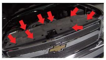
1) Open your hood and locate the (8) panel bolts. Using the panel popper tool or a flat head screw driver, gently pry the bolts free and set them aside for later. The black protective covering will now be able to be removed.
