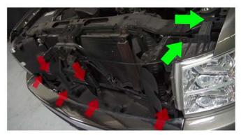
4) \*For illustration the grille has been removed\* You can now see each of the 6 mounting locations for the grille tabs that need to be pressed out in figure 3(red arrows). Once these are removed, you will now need to remove the (2) 10mm bolts holding the headlight in place (green arrows).
