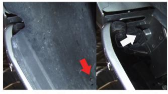
5) Before being able to full remove the headlight, you will need to locate a 10mm bolt (red arrow) in the fender well. Remove this, and peel back the liner to expose the last 10mm headlight bolt (white arrow).
