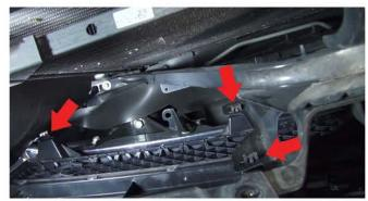
3) This is a top-down angle from above the grille, looking directly down into the radiator support and back of the grille. There 3 tabs per side for a total of 6 tabs that need squeezed and pressed out in order to get the grille free. (see fig.4 for all 6 locations)
