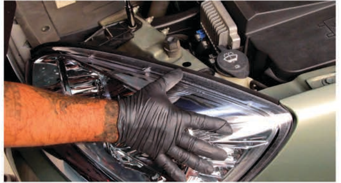
6) Reinstall [2x] 10mm bolts to mount the headlight.
