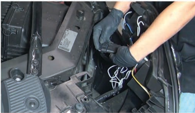
7) Connect the headlight harness to the Spyder headlight.
