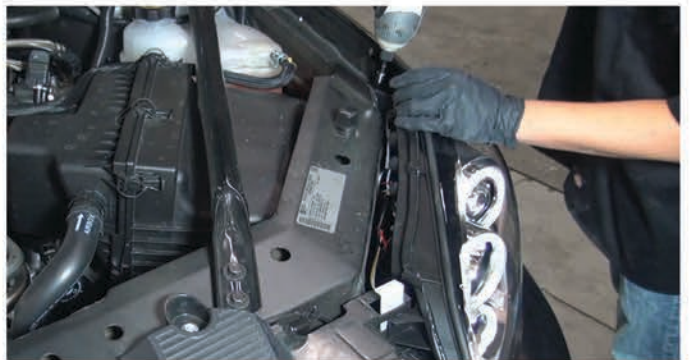
10) Reinstall [1x] 7mm bolt to secure the headlight.
