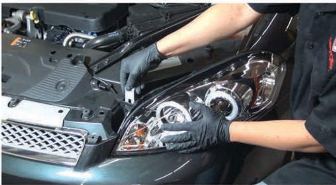
9) Reinstall [1x] plastic pull tab.
