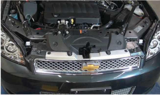
11) Reinstall [4x] Plastic retainers.
