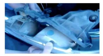
3) Unseat the headlight and disconnect the headlight wiring harnesses. Then remove the high and low beam bulbs from the OEM headlight assembly, as we must transfer these to the SPYDER headlight.
