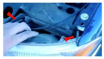
2) Rotate the two L-shaped retainer bars out of the way, then you can remove them and set them aside for now.
