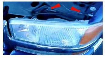
1) Open the hood. Locate the two L-shaped retainer bars that secure the headlight.
