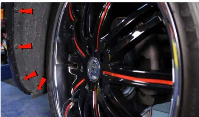
3) Remove [4x] plastic retainers securing the fascia to the fender liner.
