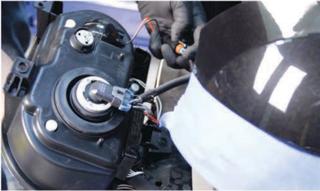
17) Reconnect the low beam and high beam harnesses.
