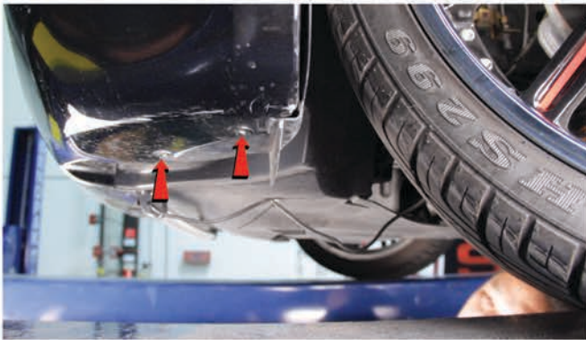
7) Remove [2x] 7mm bolts securing the bottom corner of the fascia on each side.
