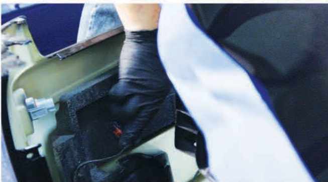
9) Disconnect the sidemarker harnesses.
