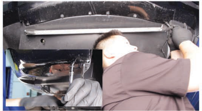
26) Reinstall [6x] plastic 7mm bolts that secure the fascia to the undertray, then reinstall [2x] 7mm bolts that secure the bottom corner of the fascia on each side..
