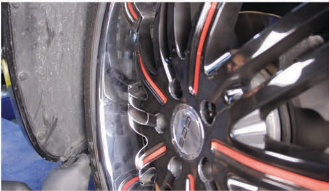
25) Reinstall [4x] plastic retainers to secure the fender liner to the fascia.
