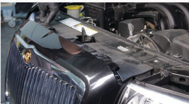
27) Reinstall [4x] plastic retainers to secure the fascia to the header panel.
