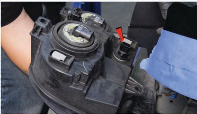
13) Disconnect the turn signal harness.
