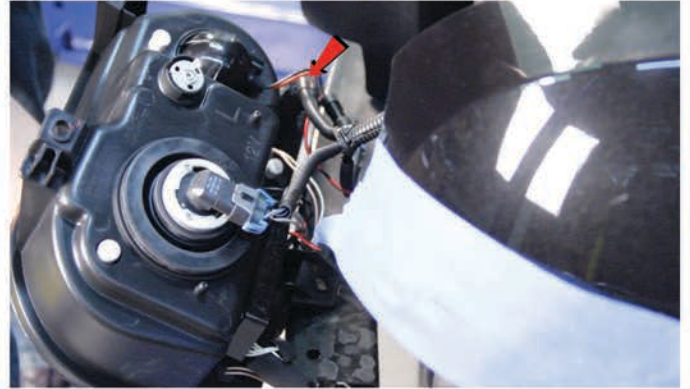
18) Reconnect the turn signal harness.
