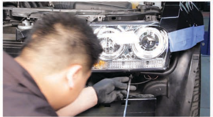
20) Reinstall [3x] 10mm (T-30) bolts to secure the headlight.
