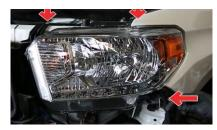
5. Remove (3x) 10mm bolts securing the headlight.
