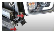
12. Install headlight garnish and reinstall (2x) plastic retainers.
