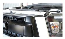
14. Reinstall (4x) 10mm bolts above the grill and (2x) plastic retainers.
