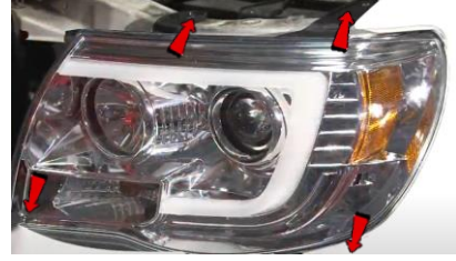
18. Reinstall (4x) 10mm bolts securing the Spyder headlight.
