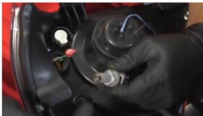
15. Remove bulb from side marker and install Spyder socket insert.
