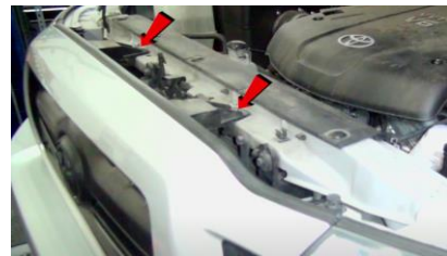
2. Remove (2x) Philips screw.
