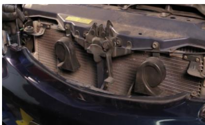
15. Reinstall (2x) 10mm bolts and (1x) plastic retainer securing the top of the bumper fascia.
