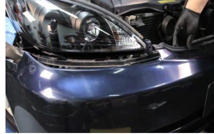
12. Seat front bumper fascia. (Reconnect fog light harnesses if equipped)
