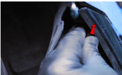
13. Reinstall (1x) 10mm bolt securing the corner of the bumper fascia.
