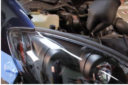
11. Reinstall (2x) 10mm bolts to secure Spyder headlight.
