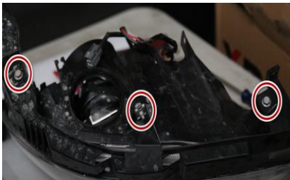
25. Remove lower bracket from OEM headlight and install onto Spyder headlight.
