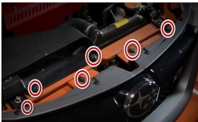
33. Reinstall (6x) plastic retainers securing the bumper and intake duct.
