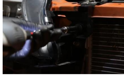
30. Install (2x) inner 10mm bolts securing the headlight.
