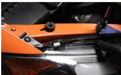
27. Reinstall (1x) 10mm bolt and (1x) plastic clip securing top of headlight.
