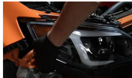
26. Seat Spyder headlight and reconnect (4x) headlight harnesses.
