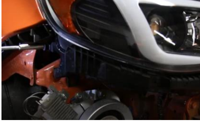
29. Install (2x) outer 10mm bolts securing the headlight.
