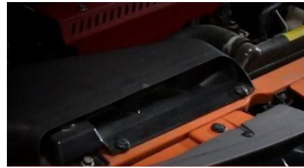
32. Reinstall intake duct.
