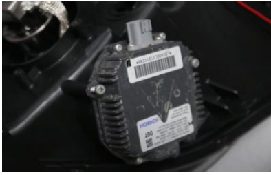
23. Install HID ballast onto Spyder headlight.
