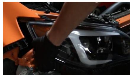
28. Seat Spyder headlight and reconnect (4x) headlight harnesses.
