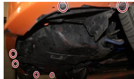
34. Reinstall (6x) retainers securing low part of bumper fascia.
