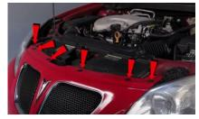
1. Remove (6x) plastic retaining clips using panel popper.
