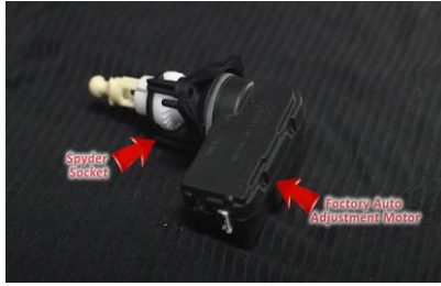
11. Finished Adjustment motor for Spyder Headlight.
