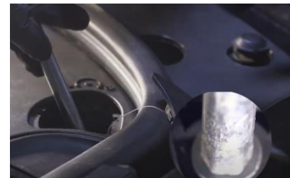
14. Using factory tool turn wrench counter clockwise to secure the Spyder headlight.
