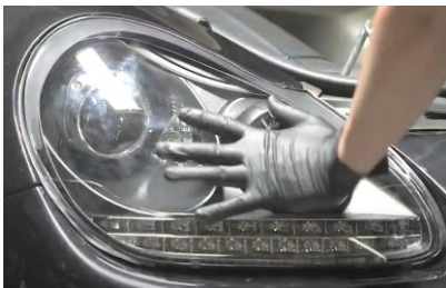
13. Seat Spyder headlight and reconnect headlight harness.
