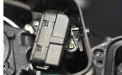
12. Install auto adjustment motor onto Spyder headlight and reinstall cover along with (6x) Philips screws.
