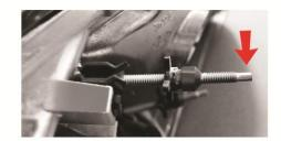
Next locate the tools that will be needed to adjust your headlamps. **Note: Please do not ever use power tools on your adjusters this may cause severe damage to the internals of your lights.**
