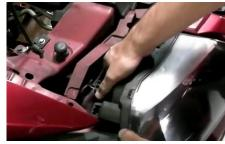
3. Remove headlight and turn signal sockets.
