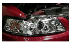
5. Reinstall side marker and headlights sockets onto Spyder headlight, next seat Spyder headlight.
