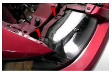
6. Install (2x) headlight retaining tabs.
