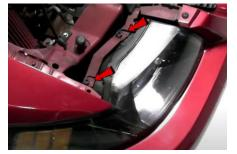
1. Pull up on the (2x) headlight retaining tabs.
