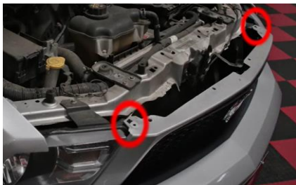
15. Reinstall (2x) 10mm bolts securing the front bumper fascia.
