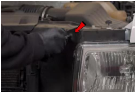
1. Remove (1x) phillips crew retainer.
