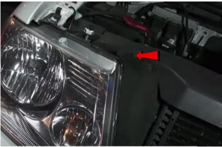
1. Remove (1x) phillips crew retainer.
