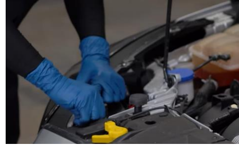
6. Reinstall (2x) T30 torx screws.
