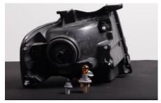
4. Remove turn signal and side marker sockets from OEM headlight (Make sure to never touch bulbs with bare hands).
