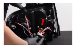
6. Install turn signal bulb onto Spyder headlight.
