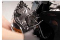
3. Disconnect Low/high beam harness along with side marker and turn signal harness.
