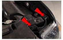
1. Remove (2x) 10mm screws securing the headlight.
