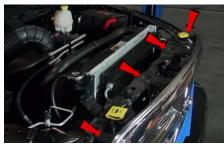
3. Remove (4x) 10mm bolts securing the grill.
