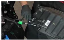
9. Remove turn signal socket and disconnect headlight harness.
