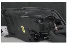
10. Remove high beam bulb from OEM headlight and install into Spyder headlight (Never touch bulbs with bare hands).
