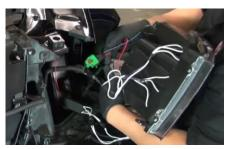
12. Install turn signal socket and connect headlight harness to Spyder headlight.
