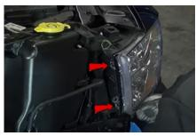
5. Remove (2x) 10mm bolts securing the headlight.
