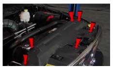
17. Replace cover panel and install (6x) plastic retaining clips.
