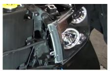
14. Reinstall (2x) 10mm bolts securing the Spyder headlight.
