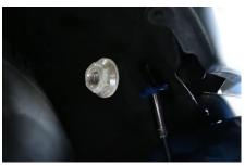
10. Reinstall (1x) 10mm behind headlight inside fender well.
