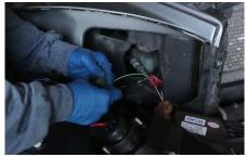
7. Connect Spyder headlight harness and install turn signal socket.
