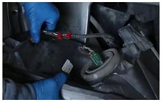
5. Remove headlight harness and turn signal socket.
