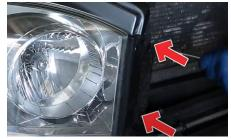
1. Remove (2x) 10mm bolts securing the headlight.
