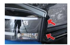
9. Reinstall (2x) 10mm bolts securing the Spyder headlight.
