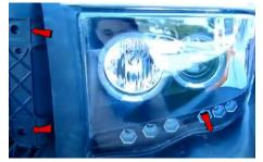
9. Reinstall (3x) 10mm bolts securing the headlight.
