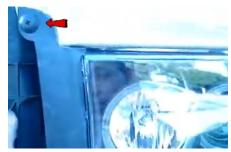
10. Reinstall (1x) plastic retaining clip.
