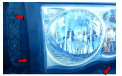
1. Remove (3x) 10mm bolts securing the headlight.
