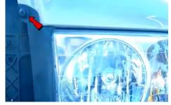
2. Remove (1x) plastic retainer using a phillips screw driver.
