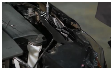
16. Reinstall (4x) 7mm bolts securing the headlight.
