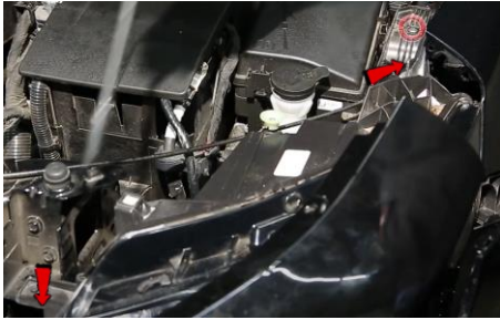
11. Remove (2x) 7mm bolts on top of headlight.
