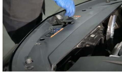
24. Reinstall (10x) plastic retainers.
