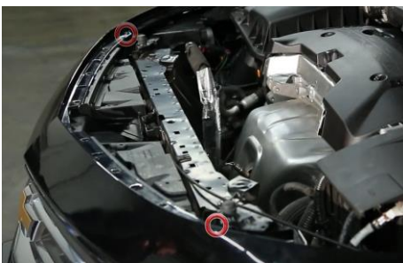
21.Reinstall (2x) T25 torx bolts.
