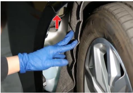
19.Reinstall (1x) 7mm bolts.
