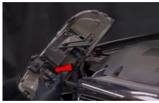
3. Remove high beam bulb by turning it clock wise (Never touch bulbs with bare hands).
