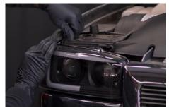
9. Reinstall (2x) rods securing the headlight.
