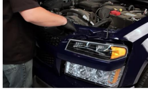
12. Seat grill assembly making sure to lock in clips.
