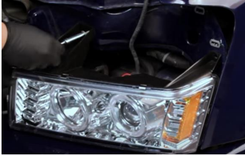
11. Reinstall (2x) 10mm bolts securing headlight.
