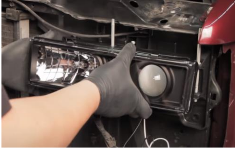
11. Seat Spyder head light and install (4x) 10mm bolts.
