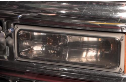
15. Seat turn signal and reinstall (4x) phillips screws.
