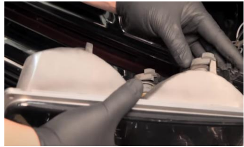
14. Install turn signal bulbs onto turn signal housing.
