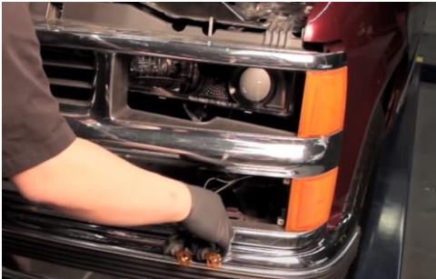
13. Make sure to carefully pull the bumper signal light bulbs through the opening.
