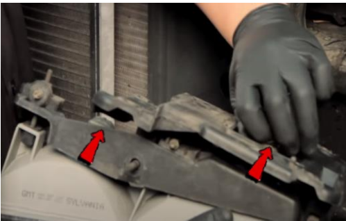
7. Disconnect high and low beam harnesses.
