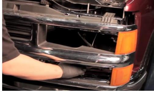
12. Reinstall corner light harness and seat the grill.
