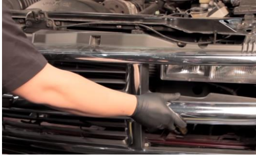
5. Unseat the grill and disconnect corner lights.
