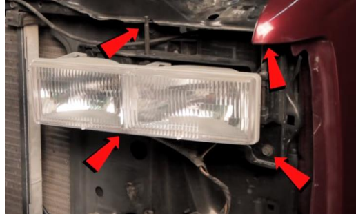
6. Locate and remove (4x) 10mm bolts securing headlight.
