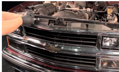
16. Reinstall (5x) 7mm bolts securing the grill.
