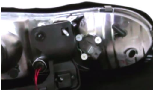
5. Install high beam bulb into Spyder headlight.
