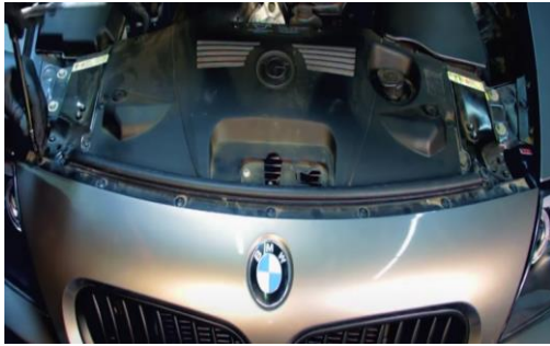
17. Reinstall hood weather strip and (7x) T30 torx bolts securing the bumper fascia.
