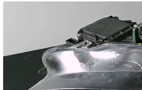
16. Transfer over AFS unit to Spyder headlight there are (4x) T20 torx screws securing it.
