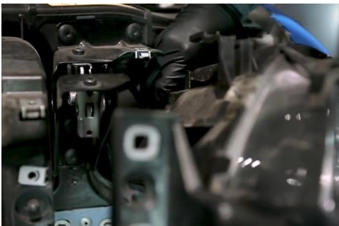
13. Disconnect headlight harness.
