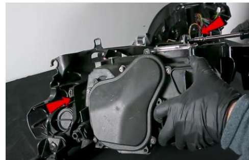
14. Remove and transfer over mounting bracket to Spyder headlight by removing (2x) T30 torx bolts.
