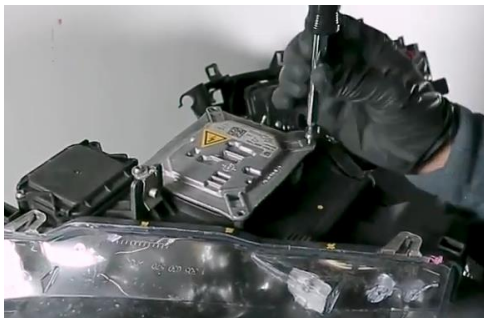
15. Transfer over OEM HID ballast to Spyder headlight there are (4x) T20 torx screw securing it.
