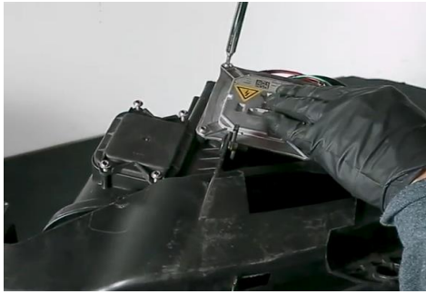
17. Secure HID ballast and AFS unit using OEM hardware.
