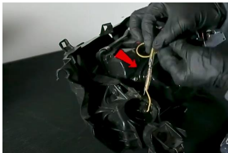
21. Connect corner light wiring.
