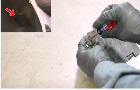
29. Reinstall fender liner access panels.
