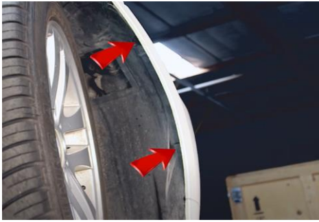
23. Reinstall (2x) 8mm screws securing fender liner on each side.
