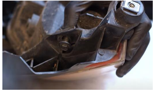
12. Remove (2x) 10mm bolts securing headlight bracket to headlight.
