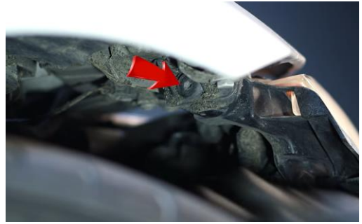
18. Reinstall (1x) T30 torx screw from behind the corner of headlight.
