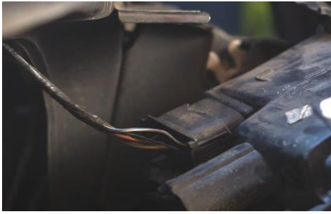
11. Disconnect headlight harness.
