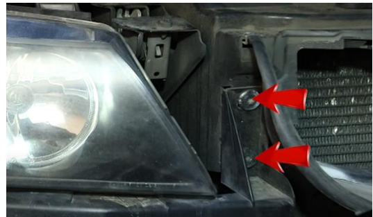
8. Remove (2x) T30 torx screw.
