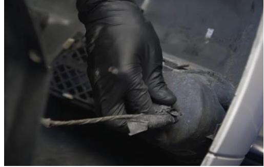
6. Disconnect both fog lamps.
