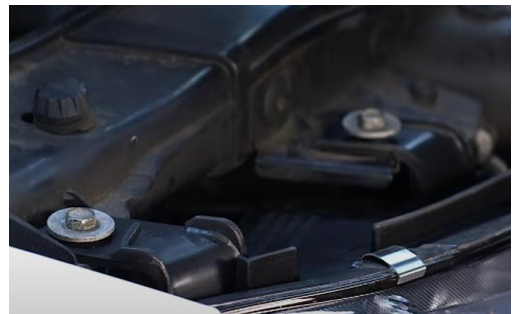
16. Install (2x) 10mm bolt on top of headlight.
