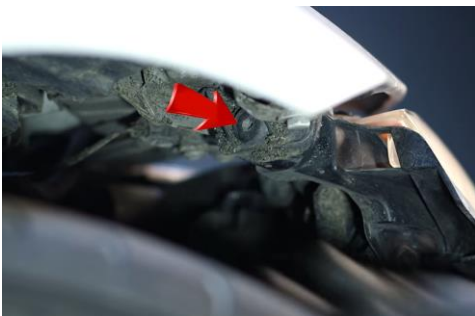
9. Remove (1x) T30 torx screw from behind the headlight corner.
