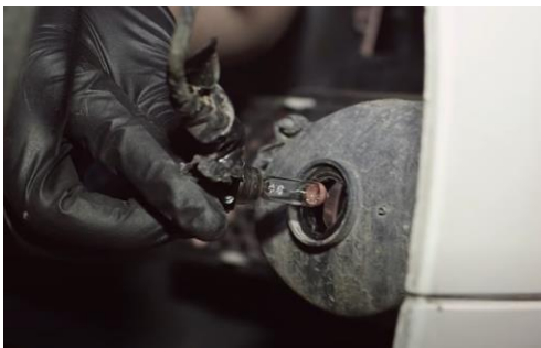
19. Reinstall both fog lamp bulbs.
