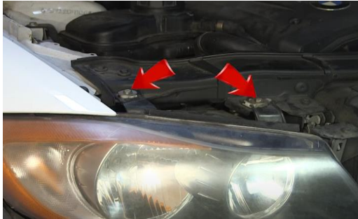
7. Remove (2x) 10mm headlight bolts.
