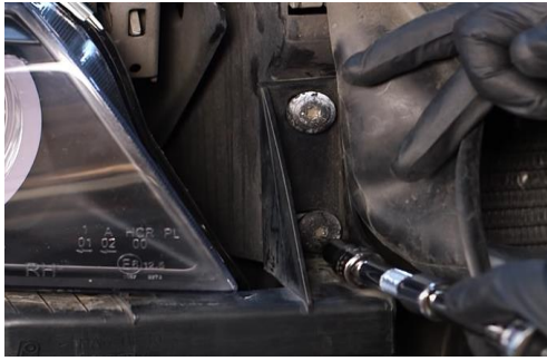
17. Reinstall (2x) T30 torx screws.
