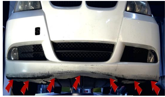
24. Reinstall (7x) screw on the bottom of the bumper fascia.
