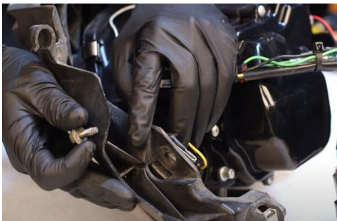
13. Install bracket onto Spyder headlight using (2x) 10mm bolts.
