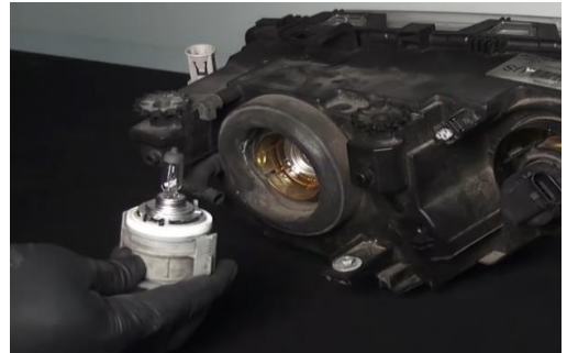
18. Remove low beam bulb from OEM headlight (Never touch bulbs with bare hands).
