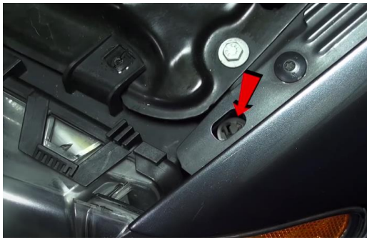
13. Remove (1x) phillips screw securing corner lamp.
