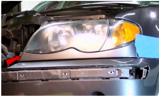
7. Under headlight remove garnish by pushing in tab and gently pull out.
