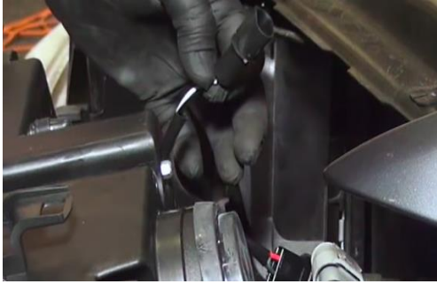
23. Black and White wire plug is only used in euro market applications.
