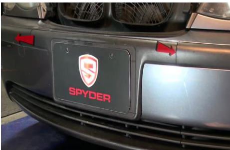
1. Gently slide bumper molding outwards.
