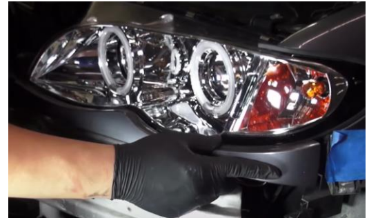
26. Reinstall headlight garnish.
