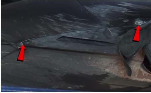
5. Remove (2x) 8mm bolts under the front fascia on each corner.
