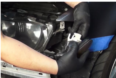
15. Disconnect corner lamp harness.
