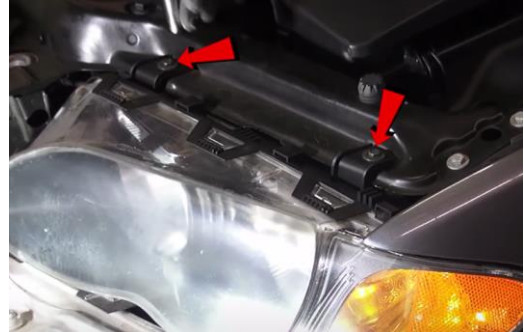
12. Remove (2x) upper 8mm bolts.
