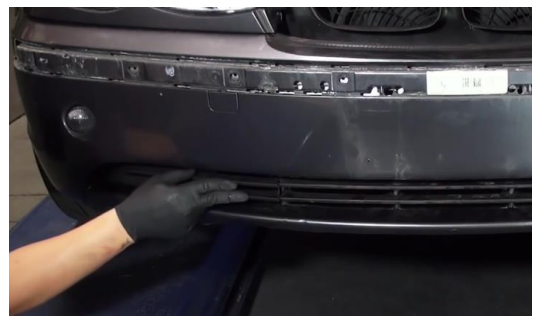
28. Reinstall both outer lower grills.
