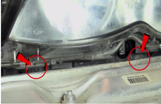
11. Remove (2x) 8mm hidden lower headlight bolts.
