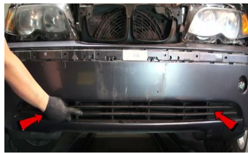
8. Remove both outer lower grills.
