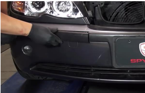
31.Reinstall both corner moldings.
