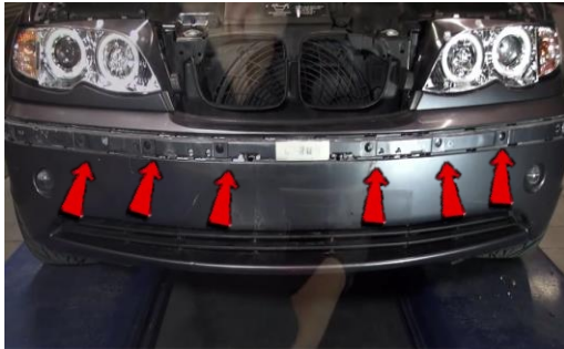
29.Reinstall (6x) plastic retainers.
