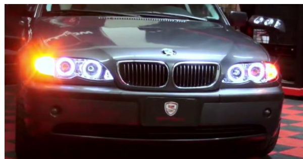
34.Turn on lights and confirm all functions are working properly. You have successfully completed the install of your new Spyder Headlights.
