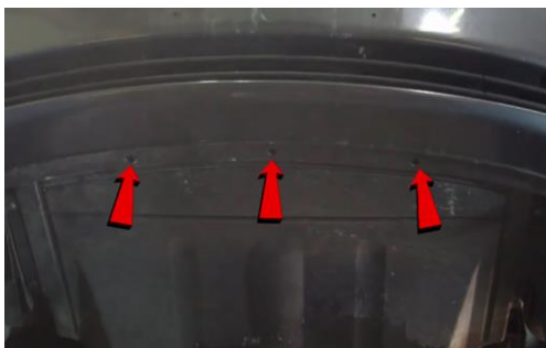
33.Reinstall (3x) plastic retainers.
