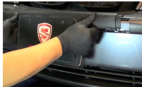
2. Remove center molding.
