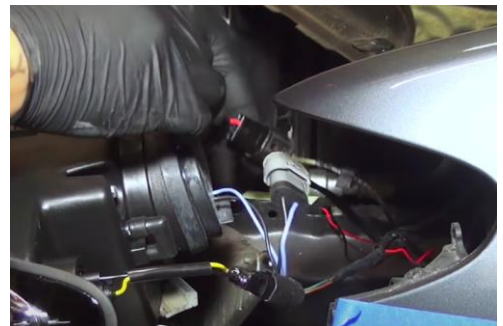
22. Reconnect the (3x) headlight harnesses.
