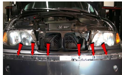
4. Remove (6x) plastic retainers using panel popper.
