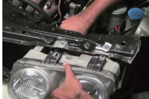
12. Remove high and low beam bulbs and remove headlight.
