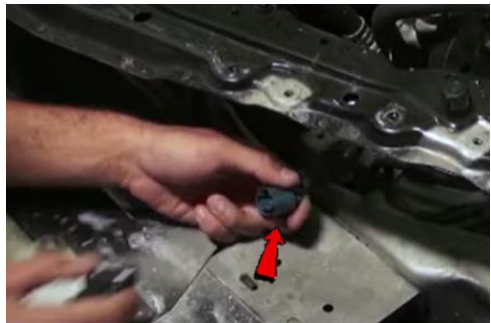
13. Remove high beam bulb from socket.
