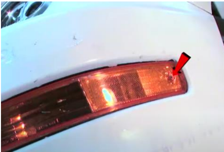
1. Remove (1x) phillips screw.
