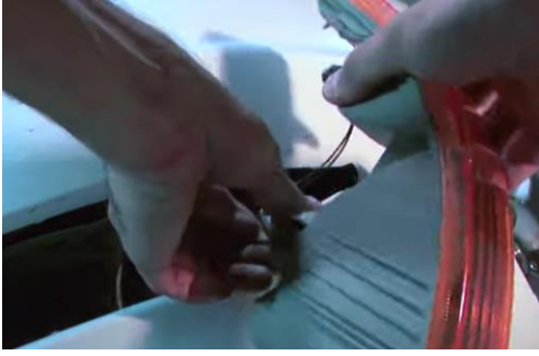
23. Reinstall turn signal sockets into corner lamp.
