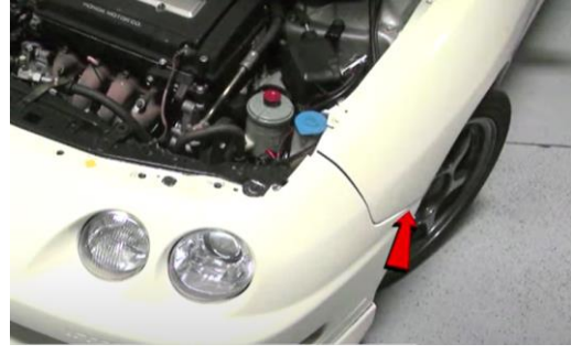
6. Remove (1x) phillips screw on each side of fascia.
