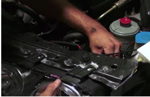
17. Insert low beam bulb.
