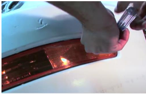
25. Reinstall (1x) corner screw securing corner lamp.
