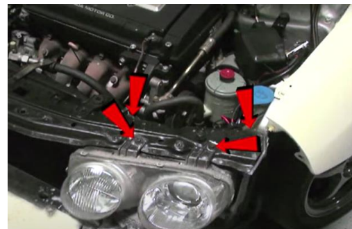
10. Remove (4x) 10mm bolts securing headlight.
