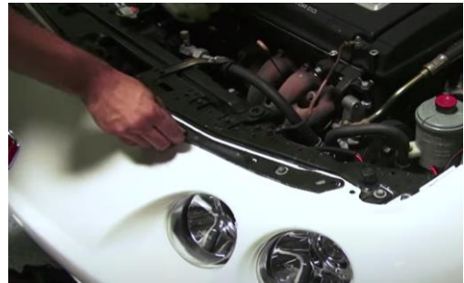
20. Reinstall support bracket and (9x) phillips screws.
