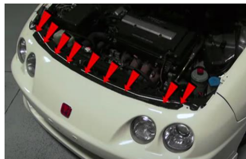
4. Remove (9x) phillips screws.
