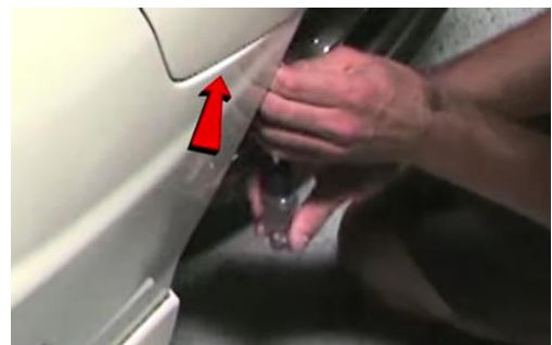
22. Reinstall (1x) phillips screw on each side of the front fascia.
