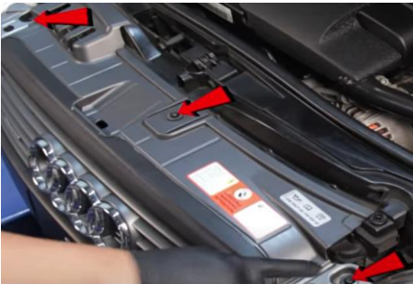
1. Remove (3x) T30 torx screws.
