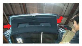
6) With the lift gate still open, using a flat head screw driver or pannel popper tool, gently pop each side of the lift gate open to reveal the second set of tail lights. Set the panels aside for later use. See figure 7 for bolt locations.
