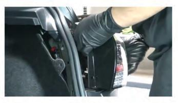
5) Attach the new harness to the OEM harness by simply snapping the plugs back together. Once this is done reseat the tail light in place, and lock down by using the thumb screw that was removed earlier. Repeat this same process for the opposite tail light.
