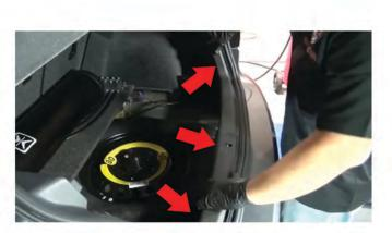
9) Once the panels have been replaced, get the U-Liner that was removed from earlier and place back into position. Make sure the trunk liner in placed under the U-Liner before snapping back into place. With a little pressure the U-Liner should pop back into its original location, and you're done!
