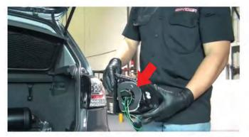
8) Now we will be reinstalling the tail light. Before remounting the tail light assembly, make sure that the gasket is in place before placing back onto the car. Place the new spyder tail light assembly back into mounting location and be sure to feed the wires through the opening. Reinstall the two 10mm bolts, then attach the harness, and replace the panel by pushing it back into position.
