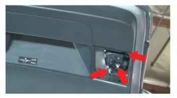
7) Once the access panel has been removed you will now be able to get to the two (2) 10mm bolts that need to be removed in order to unmount the tail light. Before completely removing from the lift gate, disconnect the harness (middle red arrow) so that the assembly can come free.
