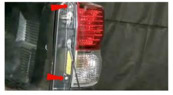
1) Open the tailgate and remove the two T30 torx screws securing each tail light.
