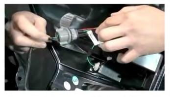
4) Connect the SPYDER tail light's wedge socket insert harness to the brake lamp bulb socket. Be sure to line up the black wires on both sides of the harness. Failure to do so can cause electrical problems and will void your warranty.
