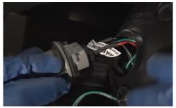
5. Install brake socket insert. (Align black wire from socket to black wire of socket insert)
